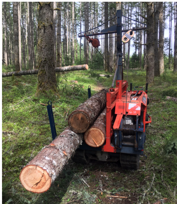
Image 10: Mobile mini cable yarder with rubber tracks allows for harvest of multiple 16-foot logs in stand thinning projects.
